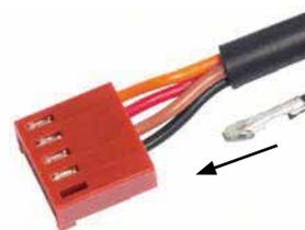
Image 2: Lock MOLEX crimp terminal of the G60-ZCTCR... cable inside connector hole of the plug.
