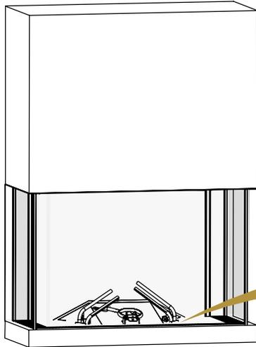
Outer bottom trim and screen must be removed to access the label, which is attached by a chain and located in a dedicated slot under the grate in the location shown above.
