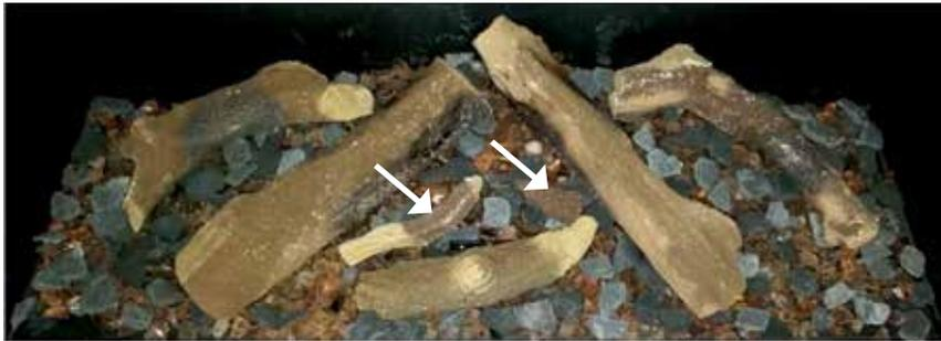
5. Position the two front small logs as shown.
