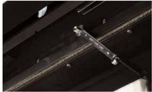
2. Remove coupling nuts from top front glass bracket using a small wrench or socket set. Remove all coupling nuts leaving the middle one until last.
