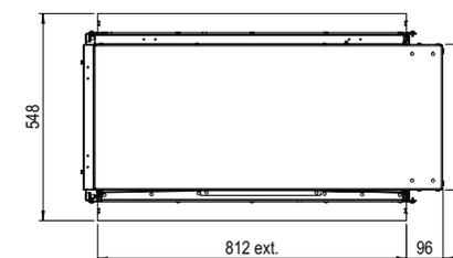
For the e-Matrix series, whilst stocks last, the fire casing may be 32mm lower than noted on the drawings in these brochures. After delivery, check the height of the fire casing to prevent misunderstandings.
